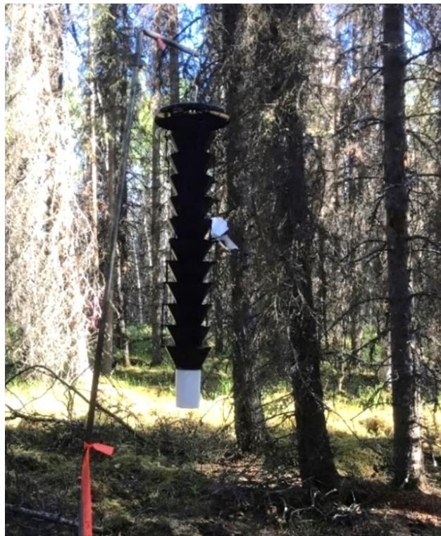
Figure 2: A 12-unit multiple-funnel trap baited with aggregation pheromones and host volatiles to assess the effects of potential inhibitors on spruce beetle near Soldotna, Alaska. Data from trapping assays are used to select inhibitors for tree protection studies. Photo by Christopher J. Fettig, Pacific Southwest Research Station, Forest Service.
